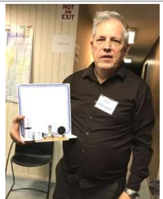
At March meeting, Earl KB5UEW brought a 20 milli watt radio he made from things he pulled from a box of old parts. The range is just 50 feet which is perfect for listening to old radio programs from his computer. The white foam core board supports the wire antenna.
