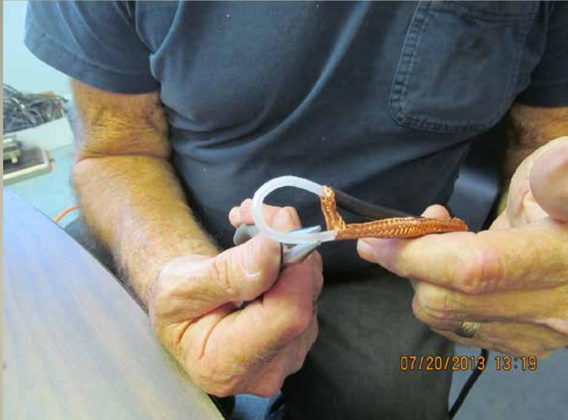
Pull the dielectric and conductor through the hole in the braid.
