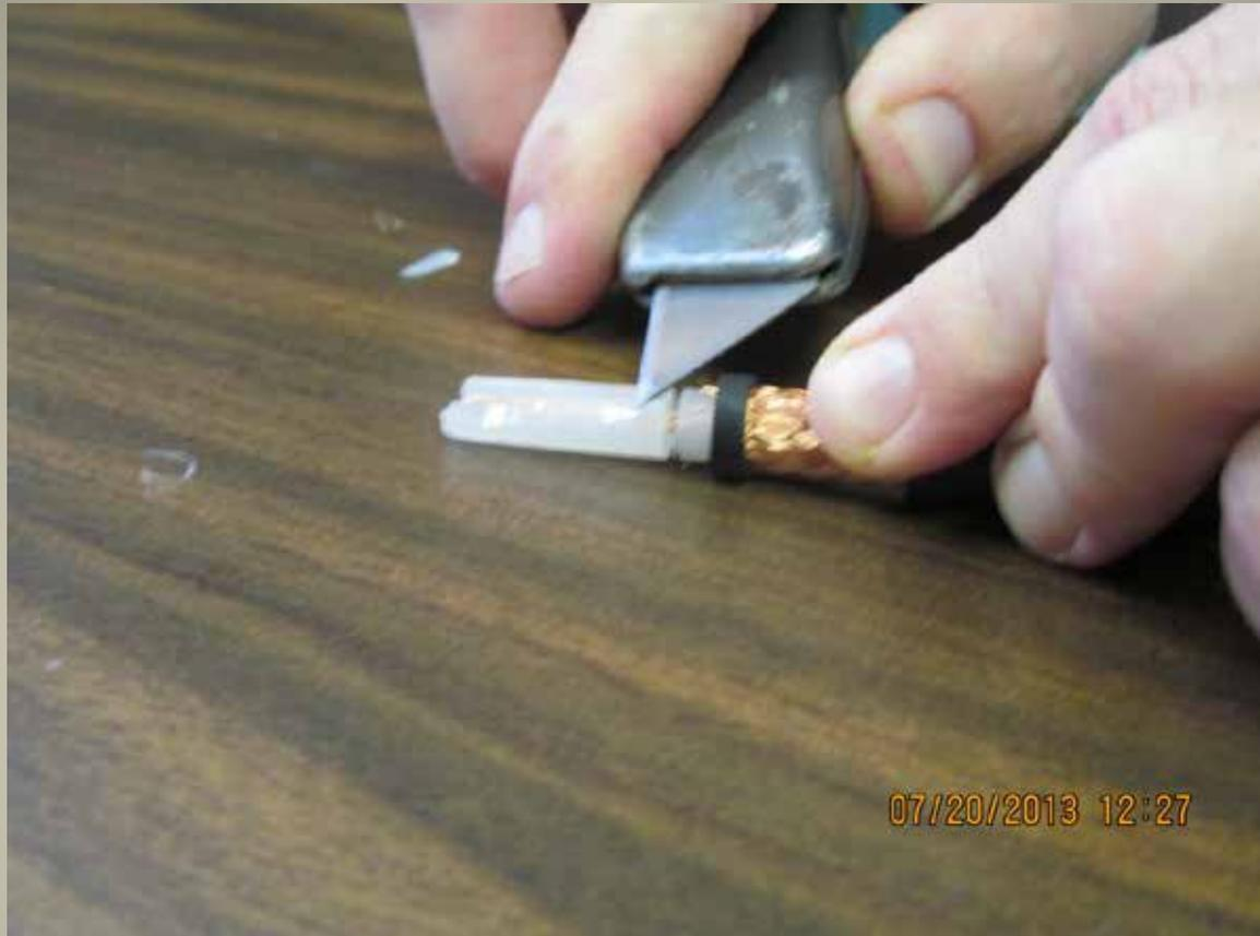
After making a circumference cut on the dielectric, it is very difficult to separate it from the conductor by pulling. Shave the plastic down to the conductor on one plane, make a lengthwise cut on the plastic, and it will separate.
