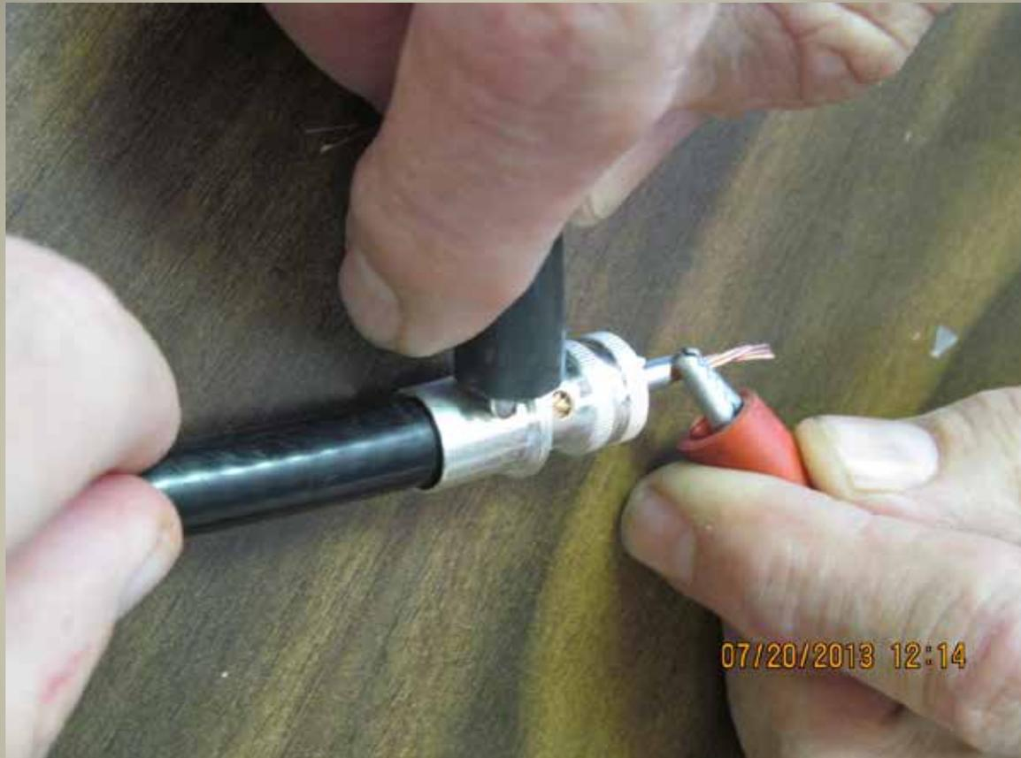
Twist the center conductor tightly and tin the conductor before installing cable in connector.
