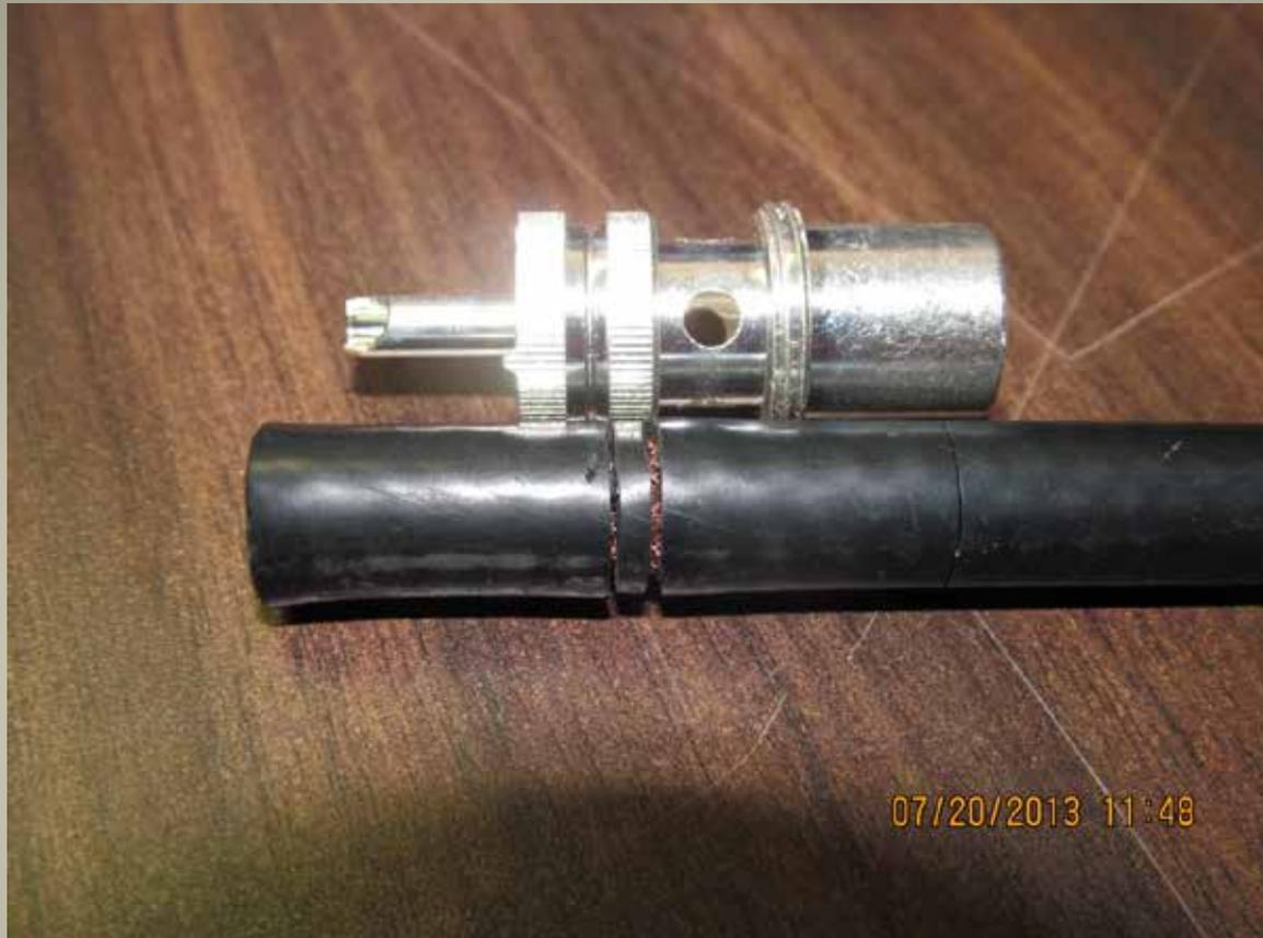
Mark all 3 cuts on the outer jacket using the connector as a guide. Allow for extra length on the center conductor, make the first 2 cuts  $1/16$ " apart on either side of the 2<sup>nd</sup> raised, knurled section, and make the third cut about  $1\ 1/8$ " from the end of the center conductor.
