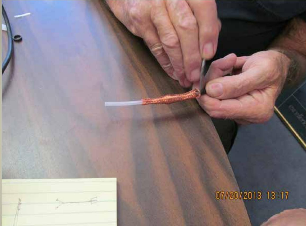
After stripping back the outer jacket, pull the braid back as far as possible.
