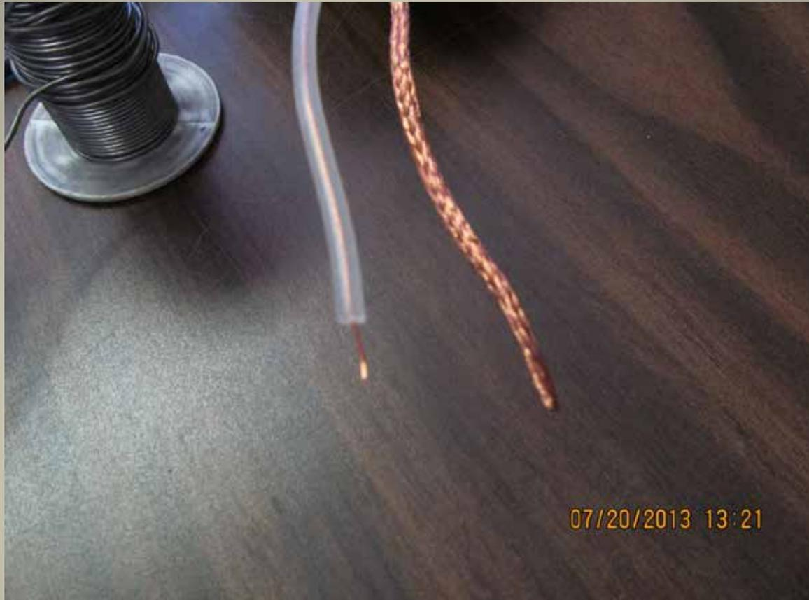
Twist the braid and strip back the dielectric. Solder or apply crimp connectors
