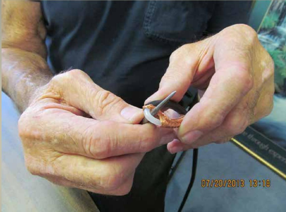
Work an opening in the braid with a pick-type tool being careful not to damage the braid.
