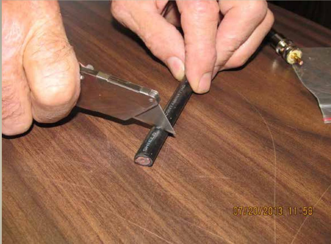
Make the cuts using a razor knife. Hold the knife with light pressure and roll the cable across the table under the knife.
