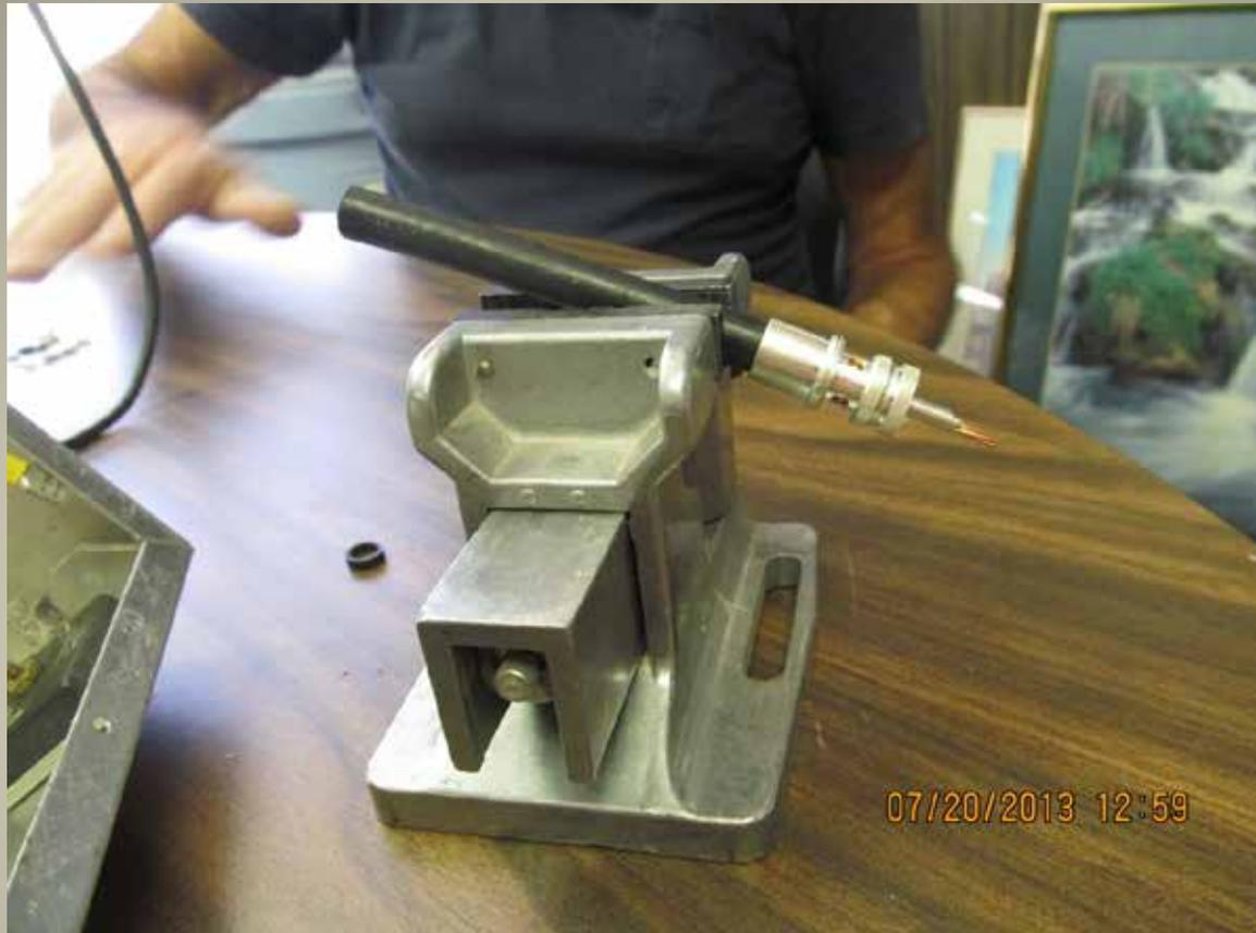
Mount in bench vise with cable and connector angled down so that solder will flow up without damaging the dielectric.
