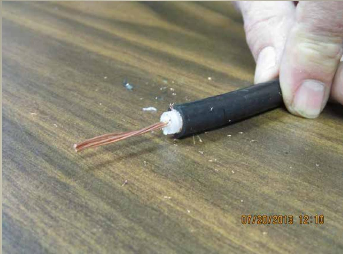
Clean up any protruding strands of the braided shield with a razor knife before removing the third length of jacket.
